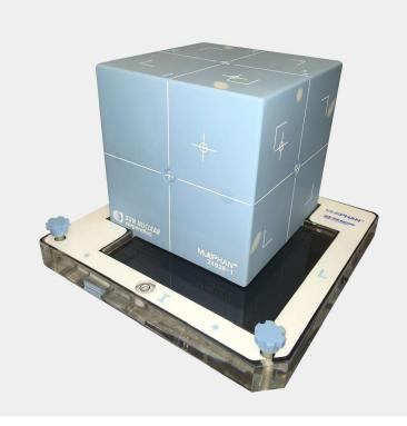
TG-142 requires confirmation that imaging system isocenters match the treatment isocenter, and that repositioning can be performed accurately. This is important to ensure that a patient, who may be imaged and repositioned with a variety of different systems, can ultimately be aligned with the radiation treatment isocenter.
