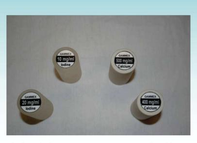
Calcium and Iodine rods of various concentrations permit easy analysis of detection ranges.
