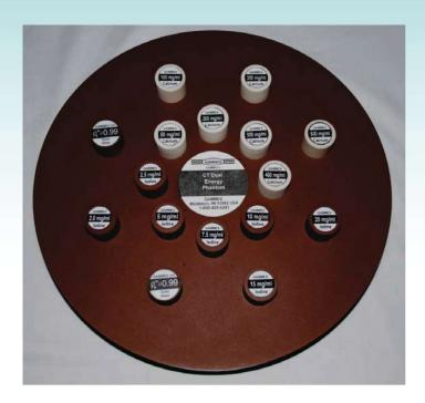
The Gammex Dual Energy CT Phantom provides users with the ability to perform Quality Assurance for Dual Energy CT analysis of Iodine and Calcium.
