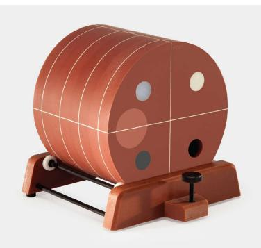
With the CT ACR 464 Phantom, you gain a multi-functional resource for your department. Not only is it essential for compliance, it allows the testing of: positioning and alignment; CT number accuracy; slice thickness; low contrast detectability, image resolution; image uniformity; spatial resolution; inter and intra plane distance measurement accuracy; and more.
