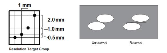
Pin targets are resolved axially if an imaginary horizontal line can be drawn between the targets without touching either target. The targets on the left are not resolved. The targets on the right are resolved.
