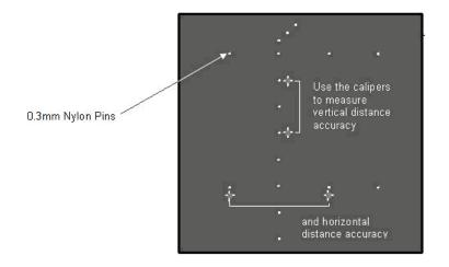
4. Freeze an image of the vertical pin targets. Use the electronic calipers to measure the horizontal width of the pin targets in the near, mid and far field of the image. Notice how the pins are narrowest in the focal zone. The pin width demonstrates the width of the ultrasound beam at that depth and approximates the *lateral resolution* of the scanner.
