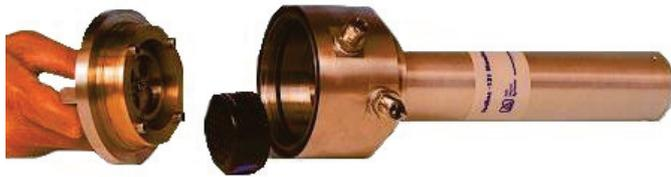
Many options exist for mounting and shielding the CGADC. With an inherent background as low as 0.1 cps, the system gives unparalleled limits of detection in most environments. However, a 2 inch shielding assembly that may be skid mounted, panel mounted or floor standing, will offer additional protection from external sources of radiation, a lower detector background and of course result quality at all times.
