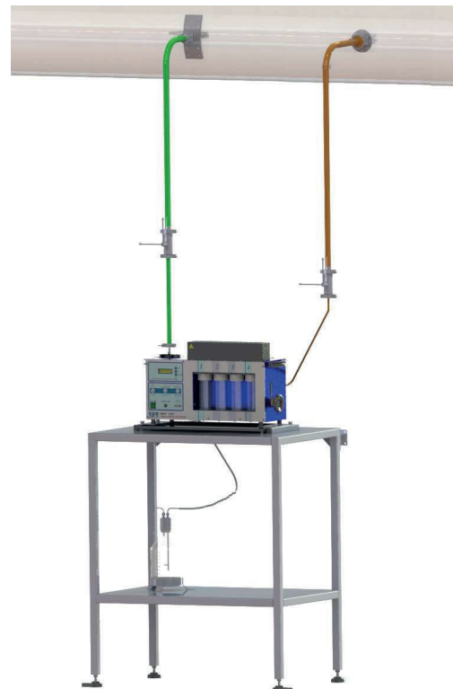
MARC 7000 installed in emission monitoring
