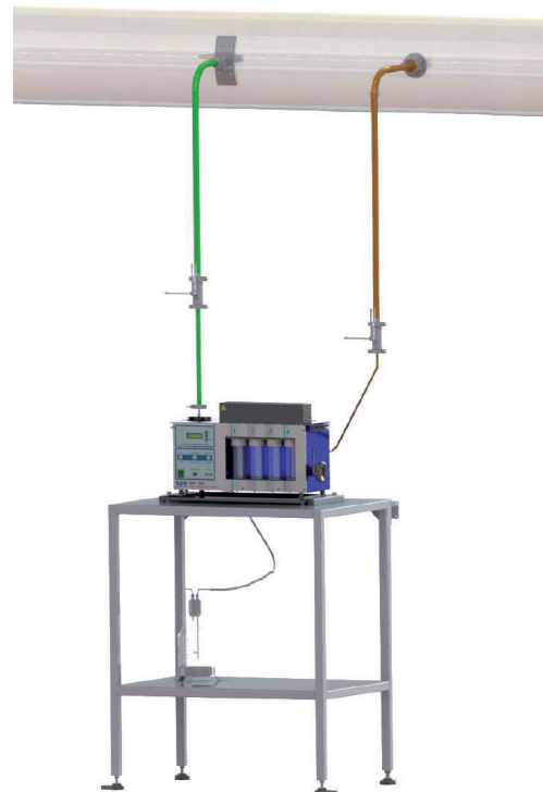
HAGUE 7000 installed in emission monitoring
