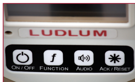
Model 9DP-1 control panel
