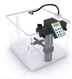
The PC Electrometer directly connects to the 1D SCANNER for monthly and annual QA.
